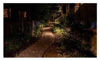
**Figure 52:** Example of path lighting using low fixtures which direct illumination downward and outward to illuminate the pathway.
