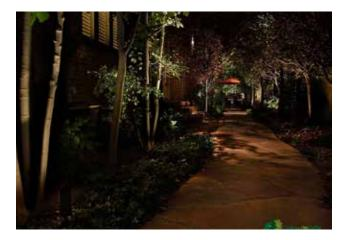
**Figure 53:** Example of lighting angled downwards to illuminate the pathway, which uses bullet type fixtures placed above the eye level on an object or tree.
